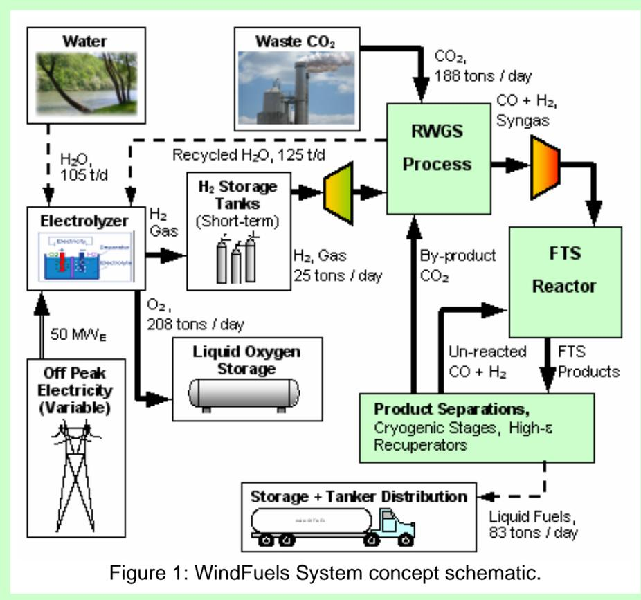
Figure 1: WindFuels System concept schematic.
